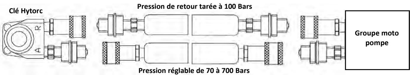
**VERIFIER QUE LES RACCORDS SONT PARFAITEMENT ASSEMBLÉS ET SERRES
